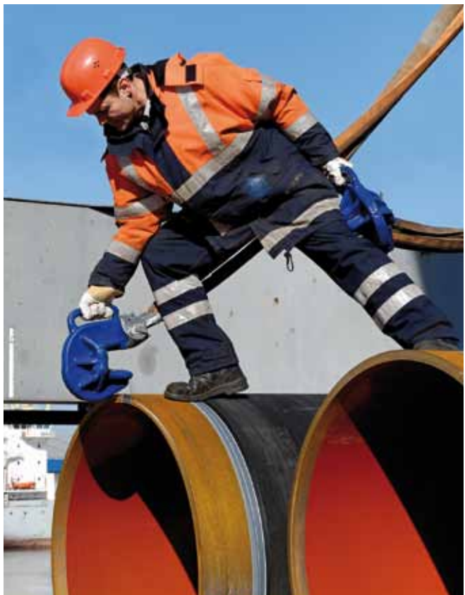
Attaching hook to steel pipes in Neustädter Hafen, Bremen
