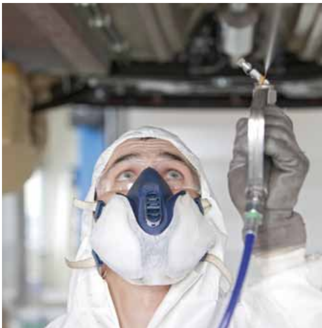
Employee wearing protective clothing while carrying out cavity sealing work on cars
